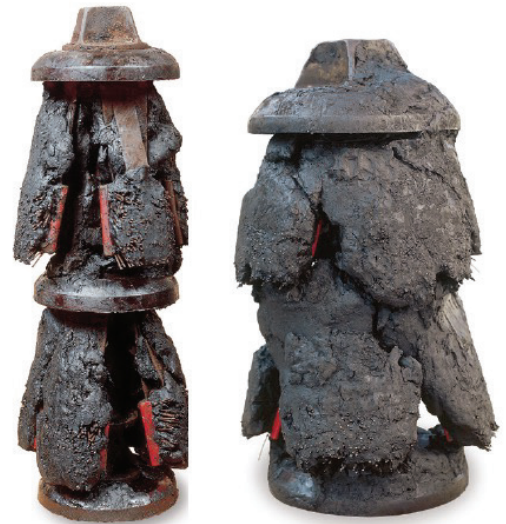
Figure 9. Lack of progressive pigging.
