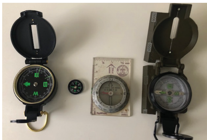
Figure 15. Compasses to assist in locating a pig or inspection tool carrying magnets.
