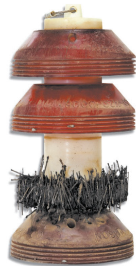
Figure 7. The effectiveness of a magnet pig.
